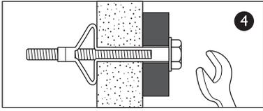
**4. Cavity Fixing - Heavy Duty wall plug:** For use when fitting or supporting heavy loads such as shelving, wall cabinets and coat racks.
