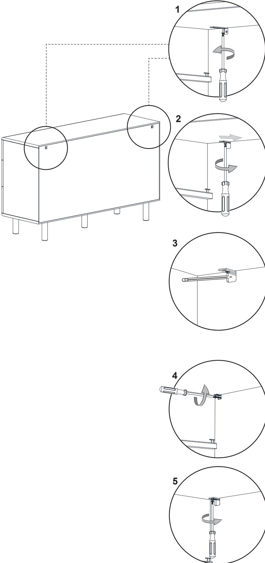
**1.** Place your product in the final position. Loosen the screws on the metal brackets just enough so that the slotted bracket can be extended to meet the wall.
