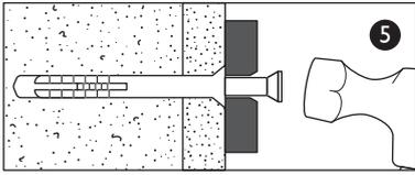
**5. Hammer Fixing wall plug:** For use with walls stuck with plasterboard. The hammer fixing allows it to be fixed to the wall rather than the plasterboard. Always check the fixing is secure to the retaining wall.
