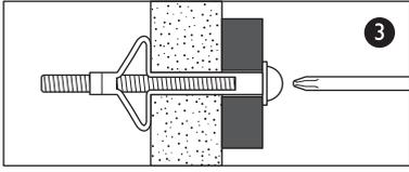
**3. Cavity Fixing wall plug:** For use with plasterboard partitions or hollow wooden doors.
