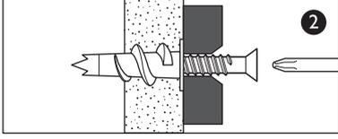
**2. Plasterboard wall plug:** For use when attaching light loads on to plasterboard partitions.
