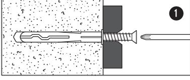
**1. General Purpose wall plug:** Generally aerated blocks should not be used to support heavy loads, use a specialist fitting in this case. For light loads, general - purpose wall plugs can be used.
