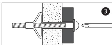
**3. Cavity Fixing wall plug:** For use with plasterboard partitions or hollow wooden doors.
