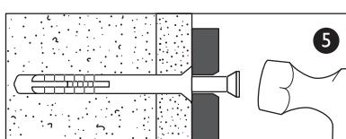
**5. Hammer Fixing wall plug:** For use with walls stuck with plasterboard. The hammer fixing allows it to be fixed to the wall rather than the plasterboard. Always check the fixing is secure to the retaining wall.
