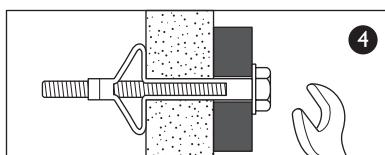
**4. Cavity Fixing - Heavy Duty wall plug:** For use when fitting or supporting heavy loads such as shelving, wall cabinets and coat racks.
