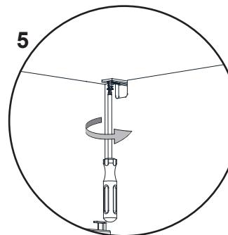
1. Place your product in the final position. Loosen the screws on the metal brackets just enough so that the slotted bracket can be extended to meet the wall.
