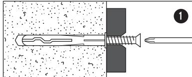
**1. General Purpose wall plug:** Generally aerated blocks should not be used to support heavy loads, use a specialist fitting in this case. For light loads, general - purpose wall plugs can be used.
